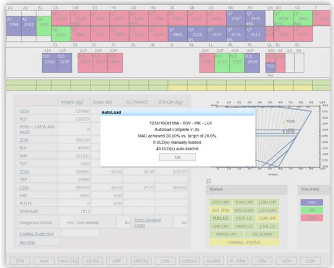
By a single click on the Auto button, the load plan is completed and a pop-up window summarizes the results. This 3-leg flight has been planned in an elapsed time of two seconds, and the target center of gravity of 28% is accomplished. The flight safety is granted as the overall status is almost fully green.
